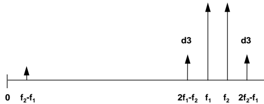
Figure 9. Two tones with in and out of band distortions
